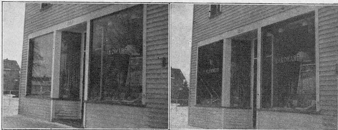
FIG. 3. — LA PHOTOGRAPHIE D'UNE VITRINE PRISE SANS INTERPOSITION D'UN ÉCRAN POLARISEUR REPRODUIT LES IMAGES QUI SE REFLÈTENT DANS LES GLACES (A GAUCHE). SI L'ON FAIT USAGE D'UN ÉCRAN POLARISEUR, CES REFLÈTS DISPARAISSENT (A DROITE)
