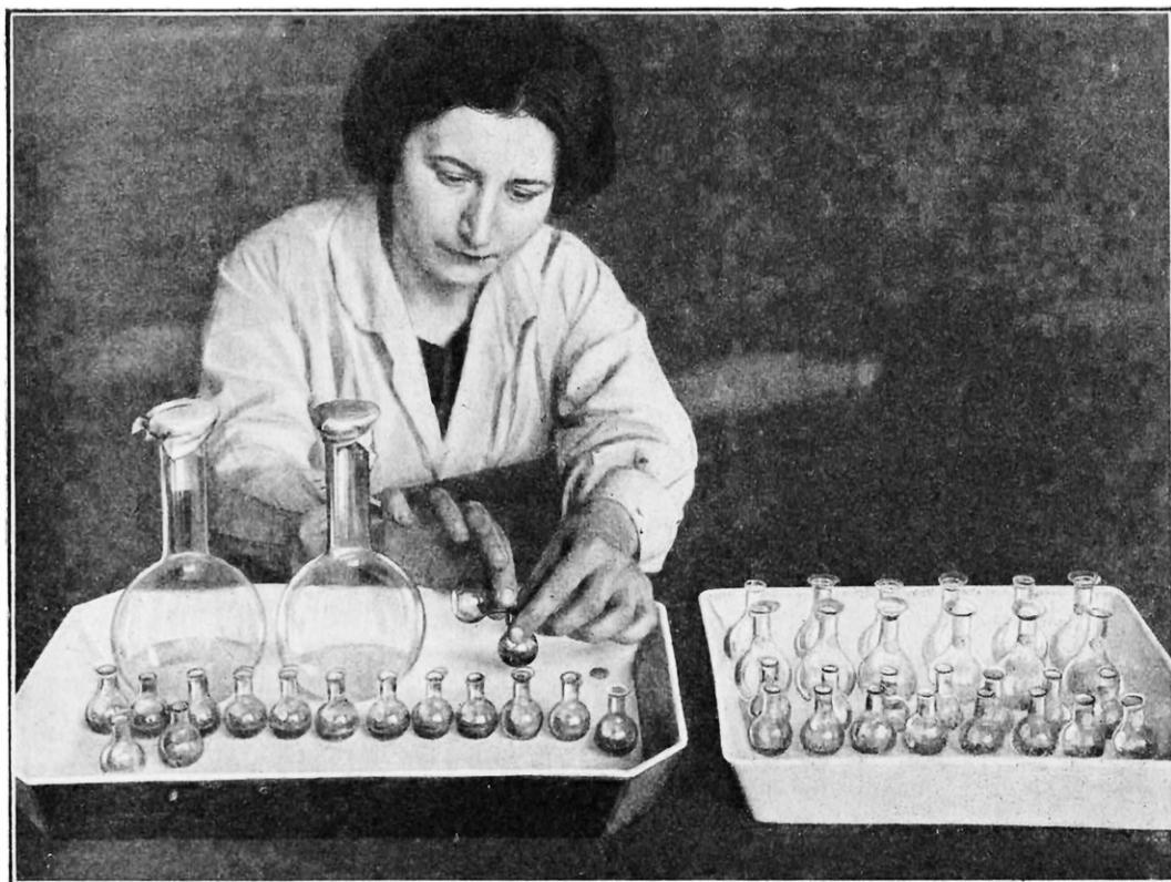
FIG. 3. — FIN D'UN FRACTIONNEMENT DE TERRES RARES
