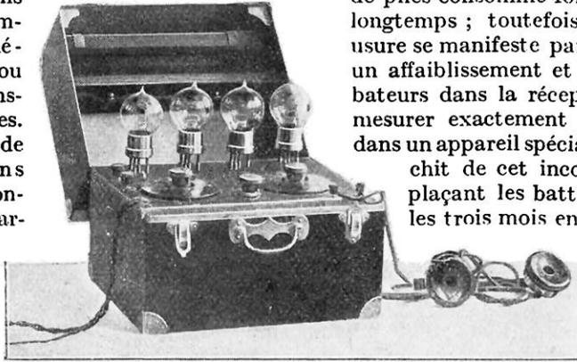
FIG. 6. — APPAREIL RÉCEPTEUR A QUATRE LAMPES, FONCTIONNANT AVEC ANTENNE
